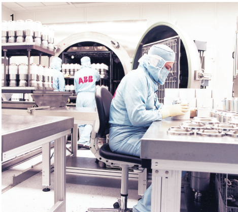
1 ABB vacuum interrupter clean room | 2 Wear indicators provide simple go / no go indication when interrupters need replacement, eliminating maintenance | 3 Integrated sensors provide required voltage and current signals for protective relaying and metering.
