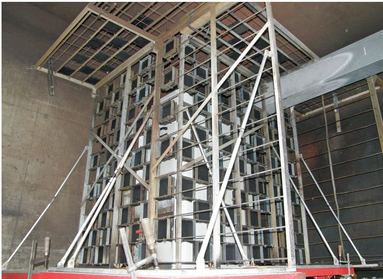
Setup for an internal arc withstand test
